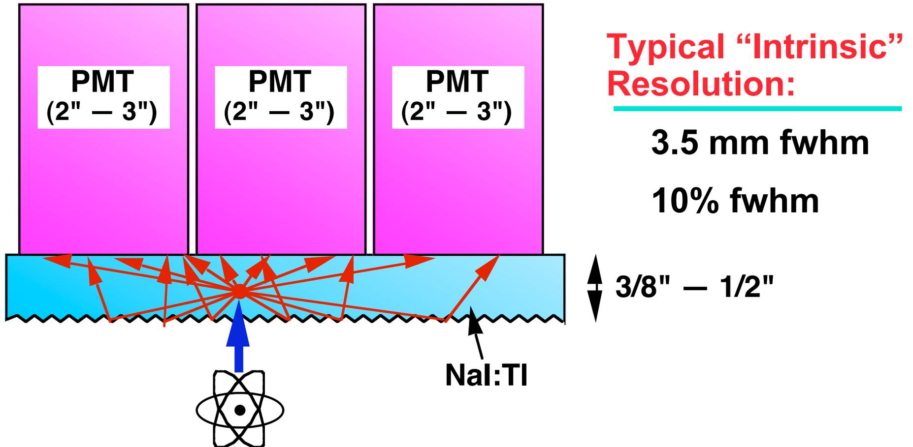
**Position Measured by PMT Analog Signal Ratio**
