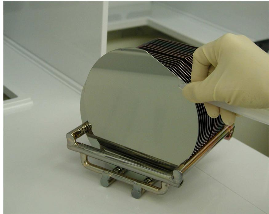
**Wafer loaded into quartz furnace boat**
