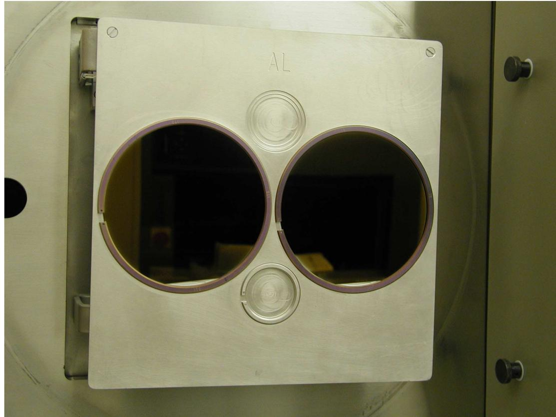
Completed ITO depositon on two 150mm wafers
