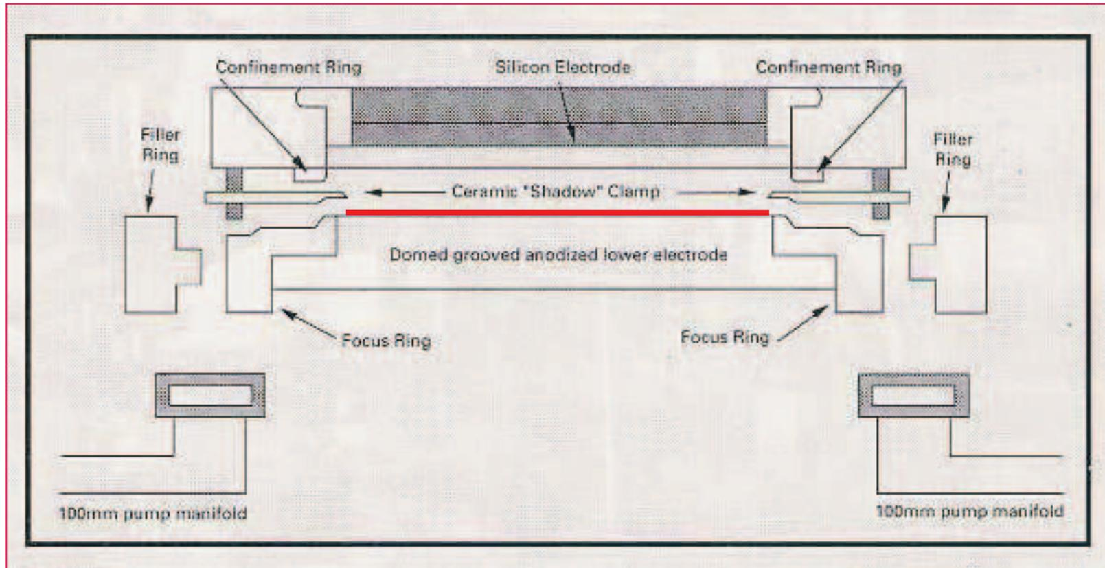
Schematic cross-section of plasma etching chamber
