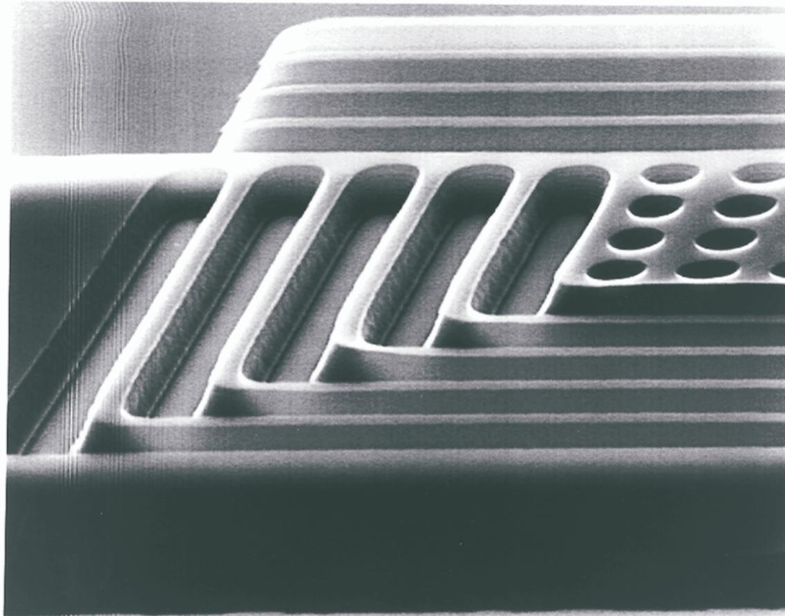
1.2 micron lines/spaces printed on the GCA wafer stepper
