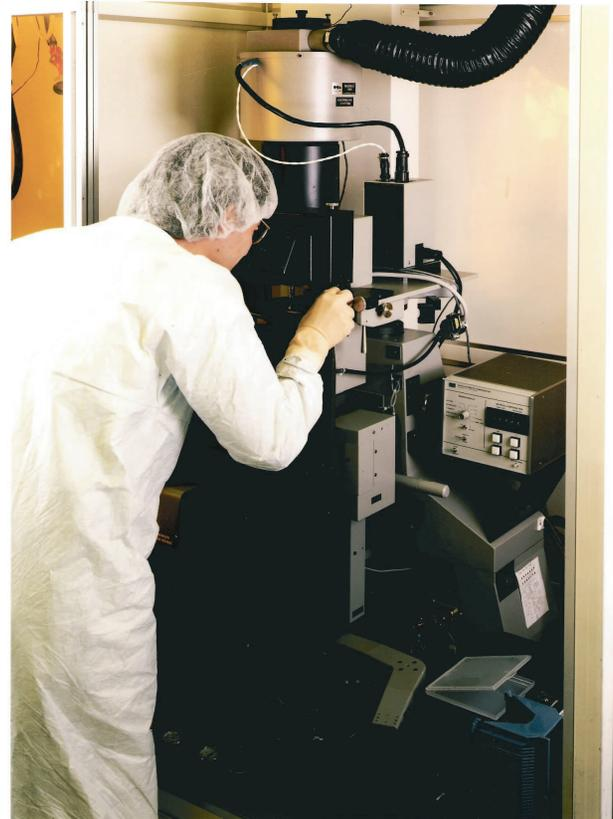
GCA Wafer Stepper – MSL's First Production Tool
