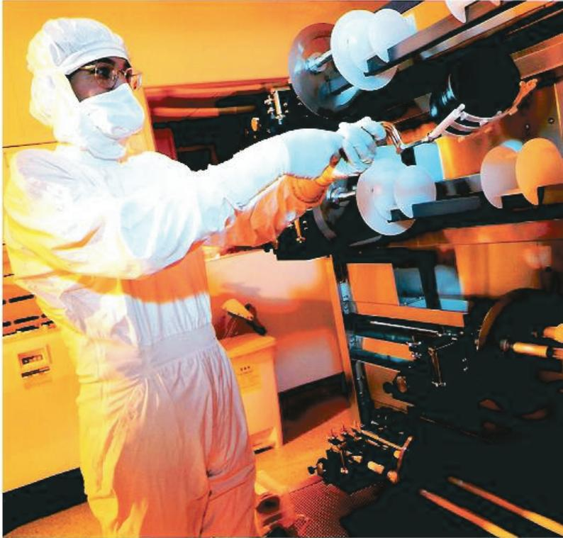
**Boat of wafers being loaded**
