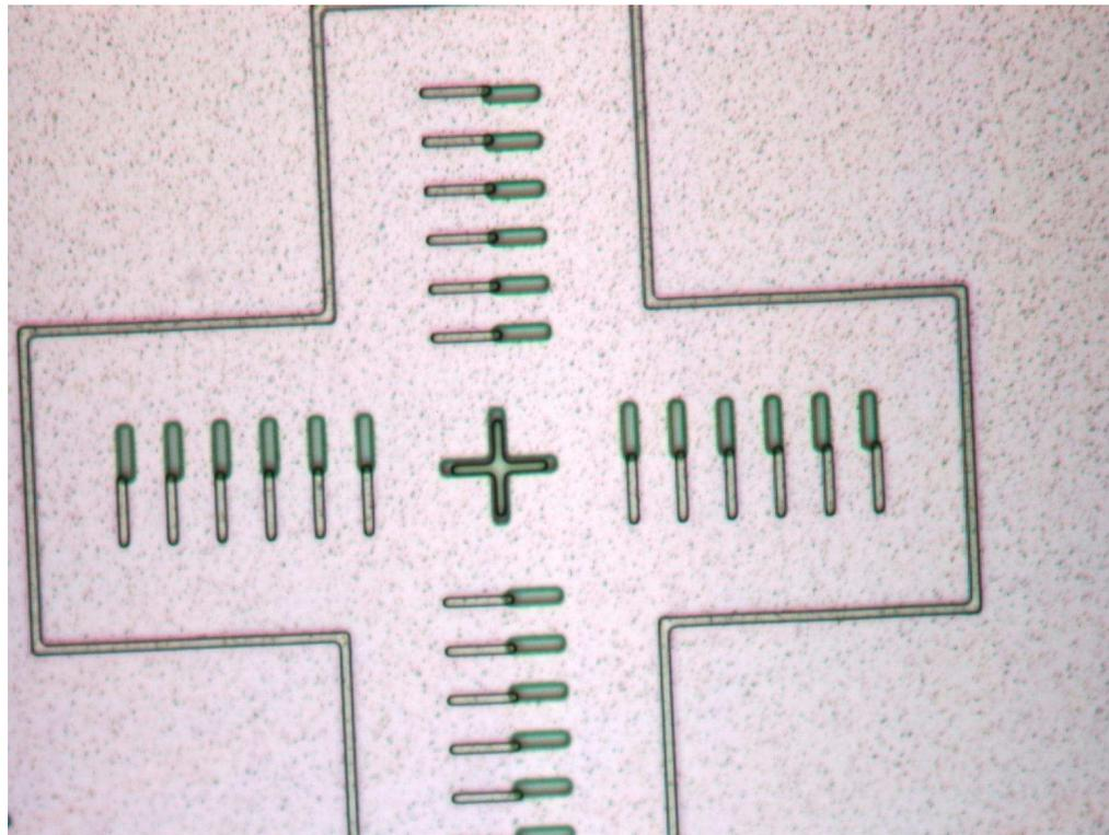
Resist pattern aligned to existing pattern on wafer
