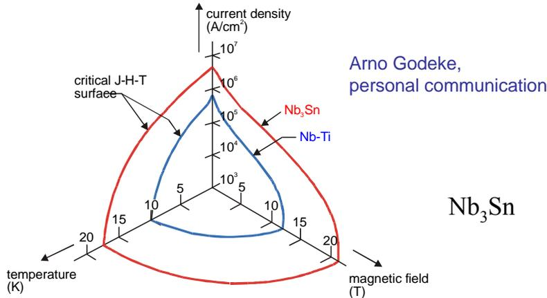
*Note: High temperature superconductors (HTS) and existing versions of MgB<sub>2</sub> do not (yet) carry sufficient current, at any temperature, to compete with PM undulators*
