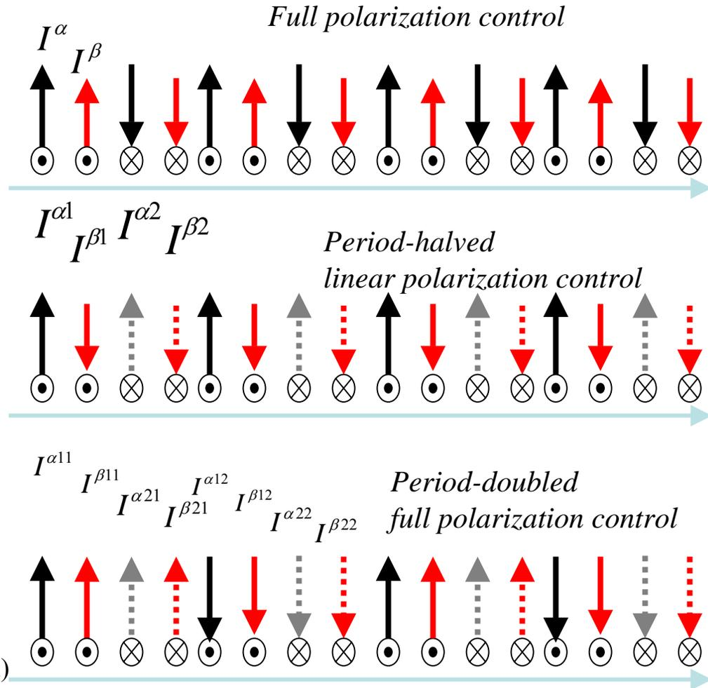
**NOTE:** Two power supplies (A, B) needed for linear polarization control; four needed for full (linear+elliptic) polarization control; switching network could provide access to the above regimes
