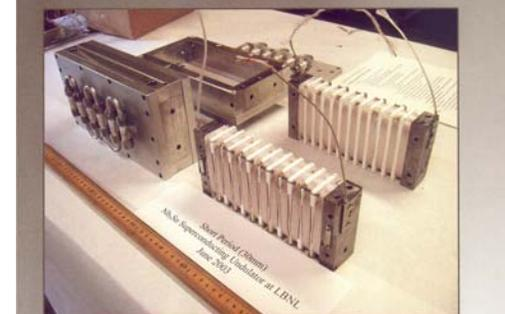
ALS SCU Superconducting Undulator at LBNL
