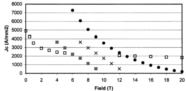
Fig. 5. Critical current vs. field for high field superconductors—Bi-2212 (open squares), Nb<sub>3</sub>Sn (triangles), NbTi at 4.2 K (solid squares), and NbTi at 1.8 K (crosses). The crossover for Bi-2212 and Nb<sub>3</sub>Sn is about 13 T on the basis of  $J_c$ . However, the practical crossover is still higher, due to the large volume fraction of Ag matrix required in the fabrication on the Bi-2212 wire at present.
