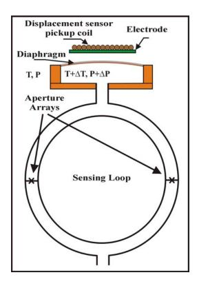
Rotation induces a phase shift between the two aperture arrays. This leads to interference at the microphone.
