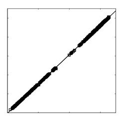
Amplitude fluctuation noise seems  $\sim 10^{-3}$ ! Thermal fluctuations seem suppressed by 1/N where N=4225.
