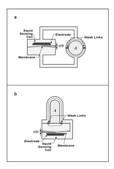
The effective critical current of the entire device is modulated by the rotation flux threading the ring (see Feynman vol 3 chap 21)
