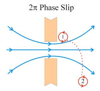
Superfluid accelerates until reaching a critical velocity at which a (thermally activated) phase slip occurs.
