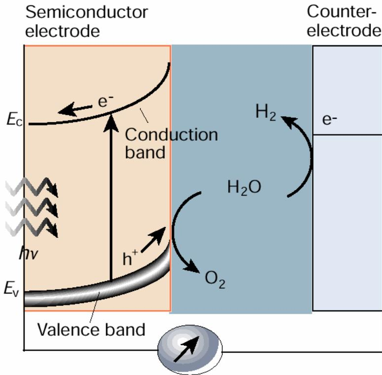
1. Absorption of light near the surface of the semiconductor creates electron-hole pairs.
