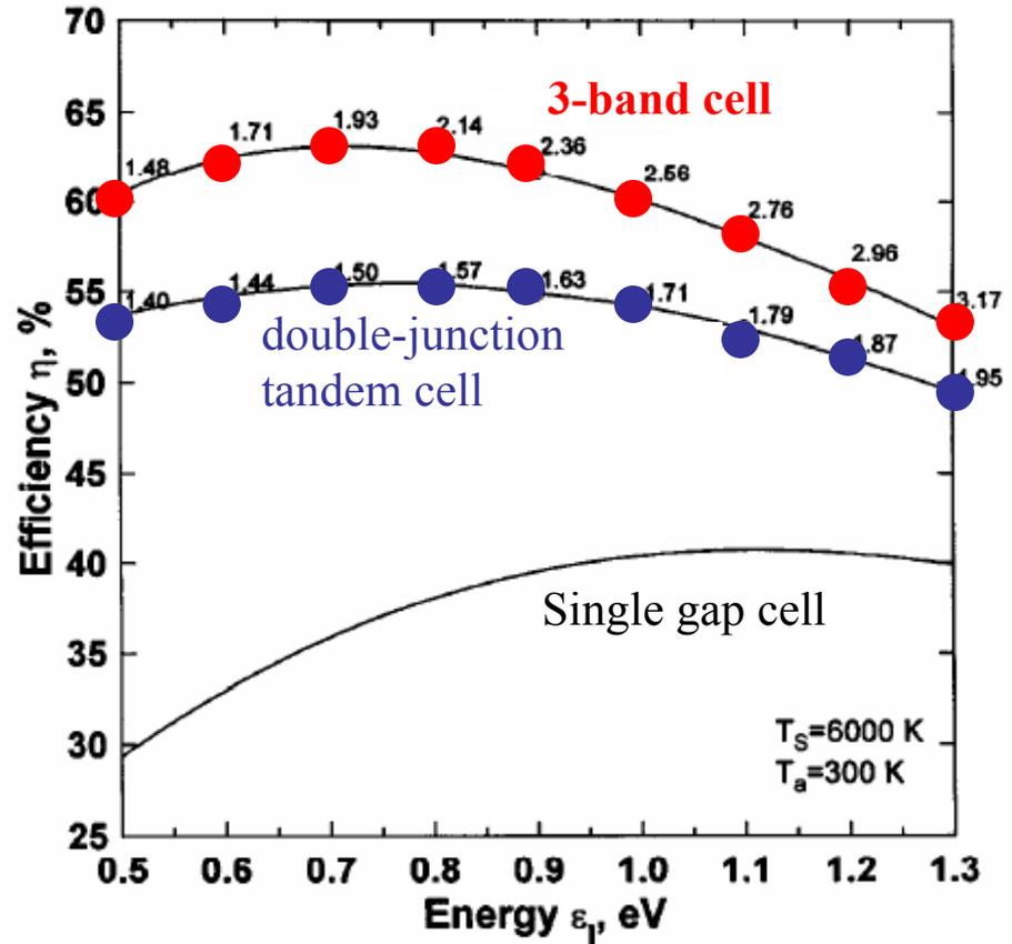
FIG. 2. Efficiency limit for a solar cell with an intermediate band and for a two-terminal ideal tandem cell, in both cases vs the lowest band gap  $\epsilon_1$ , and for a cell with a single band gap. The corresponding values of the highest band gap in cells with intermediate band ( $E_G$ ) and in tandem cells ( $E_C$ ), for maximum efficiency, are also presented.
